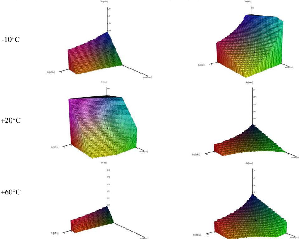
Fig. 5. The examples of compatibility subspaces, determined with ANCOMP program for epoxy (EP) and polyurethane (PU) coatings at different service temperatures, defined by compressive strength of concrete  $f_{c}$ , maximum crack width  $w_{max}$  and crack width changes  $\Delta_w$
