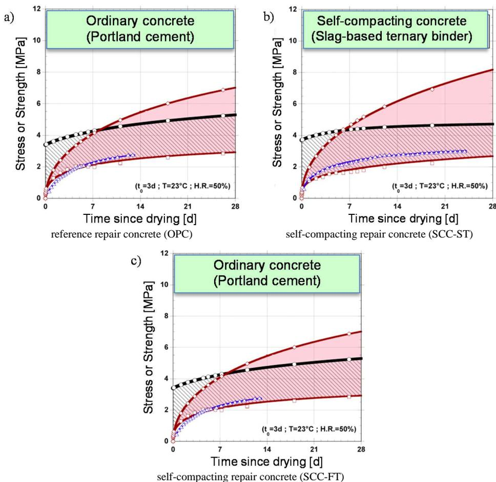
Fig.2. Comparative development of recorded and theoretical tensile stresses in AASHTO PP34 ring test specimens exposed to drying at 50 % R.H. at the age of 3 days (note: solid blue line: stress recorded in the ring; lower and upper solid red lines: theoretical average concrete stress, with and without stress relaxation respectively; solid black line: tensile strength of the concrete)
