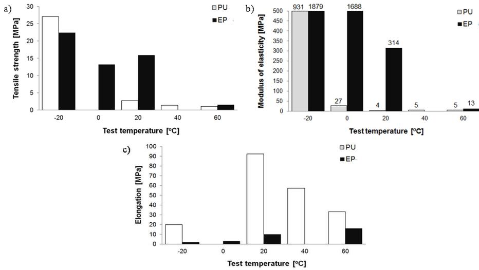
Fig. 4. Influence of ambient temperature upon a) tensile strength, b) modulus of elasticity, and c) elongation for polyurethane-based (PU) and epoxy-based (EP) coatings (test parameters: temperatures of -20, 0, 20, 40 and 60°C; deformation rate of 50 mm/min) – acc. to [8]
