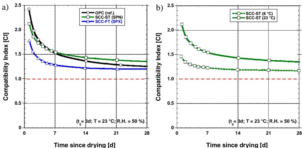
reference repair concrete (OPC) self-compacting repair concrete mixtures (SCC-ST, SCC-FT) exposed at 23°C
