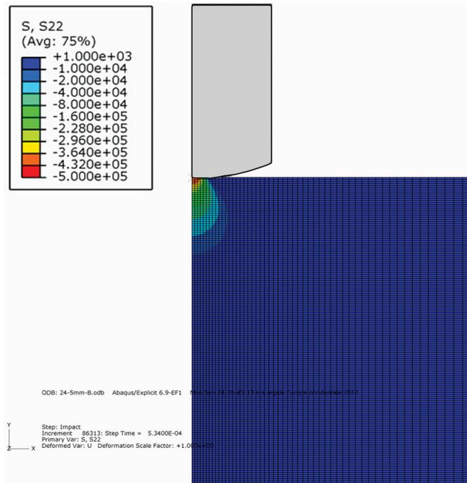
Fig. 1. Typical distribution of vertical normal stresses in concrete during the rebound hammer impact obtained by means of FE analysis. Stresses at the beginning of the contact
