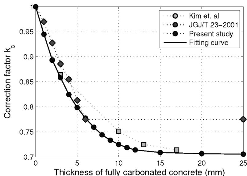
Fig. 3. Comparison between experimental and numerical values of  $k_c$
